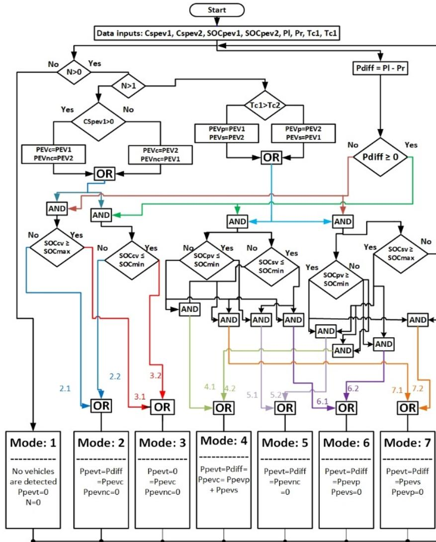
Fig. 16. Adaptive supervision system of PEVs powers [26].
