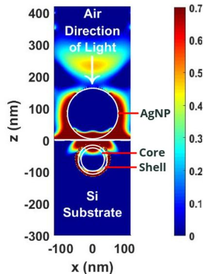
**Fig. 5.** Optical nearfield enhancement as a result of incorporating homogenous plasmonic NP on top of the substrate and a plasmonic core-shell NP embedded inside the substrate, in “sandwich” configuration.
