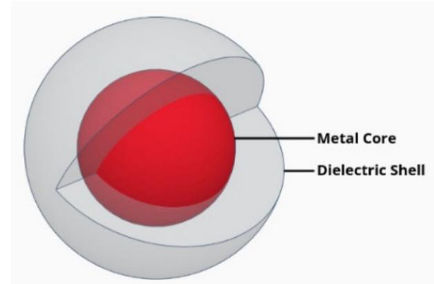
Fig. 2. Meta core-dielectric shell nanoparticle composition.
