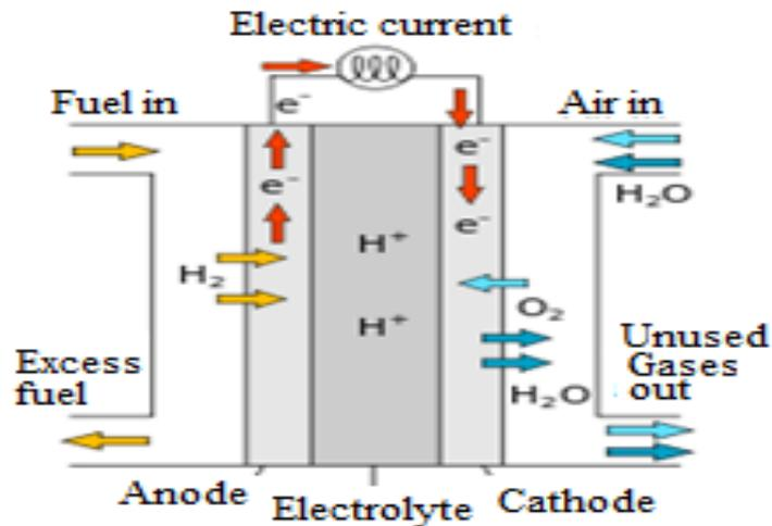
**Fig. 18. Basic structure of fuel cell system [28].**
