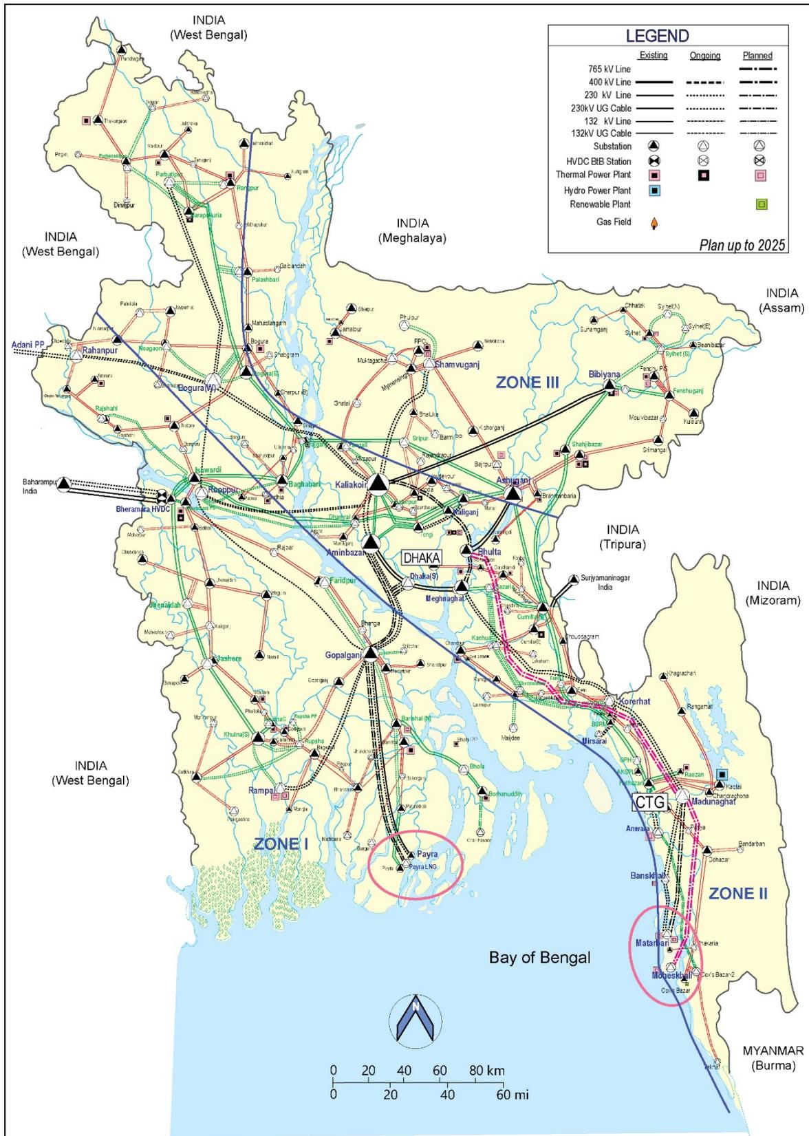
**Fig. 3. Map of the Power Grid Plan 2020-25 of Bangladesh [67]. The three earthquake zones are marked (solid blue lines) on top of the map to show the spatial distribution of the power grid infrastructures. Red ellipses mark the three under construction power hubs [65] in which in Matarbari and Maheshkhali located in the south-east, and Payra is located south-west of the map.**
