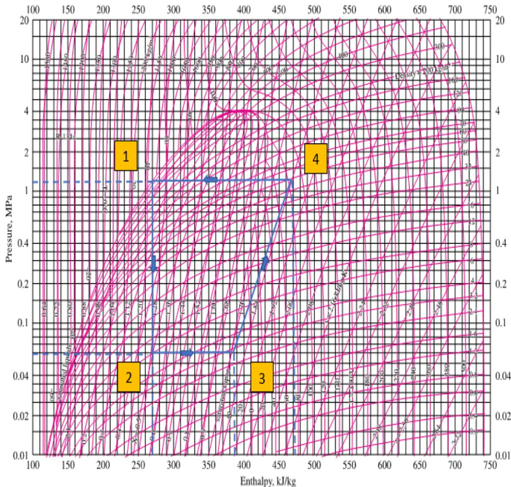
**Fig. 7. Pressure versus enthalpy diagram for refrigerant R134a.**
