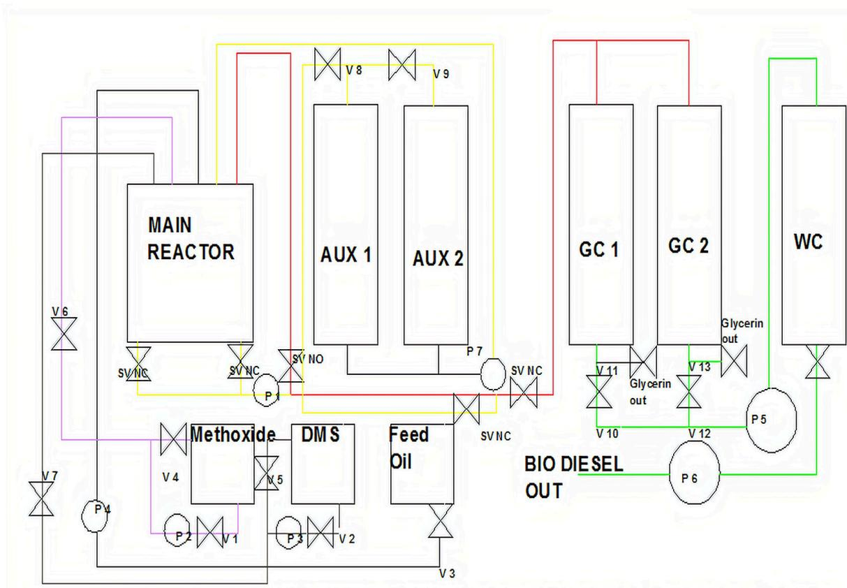
Fig. 3. Biodiesel production experimental set-up for small batch (10-25 liters/batch).
