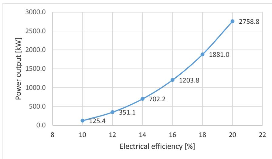
**Fig. 2. Power output as function of electrical efficiency.**
