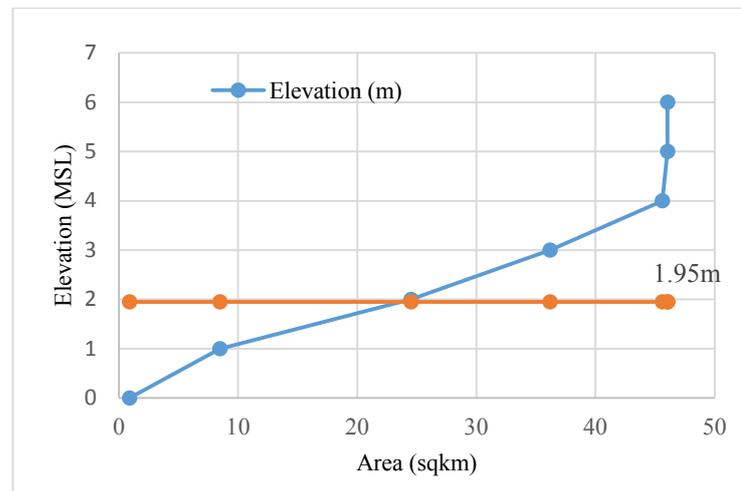
**Fig. 9. Area elevation curve for Khulna City.**
