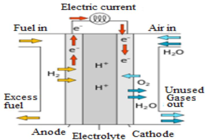
**Fig. 18. Basic structure of fuel cell system [28].****Table 4. Fuel cell specifications.**
