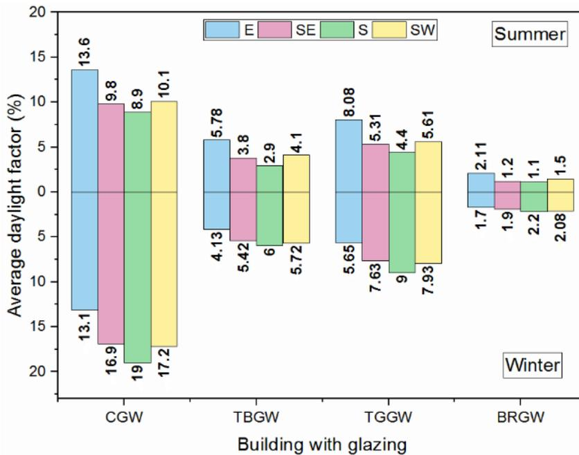
Fig. 9. Average daylight factors of various window glazing.
