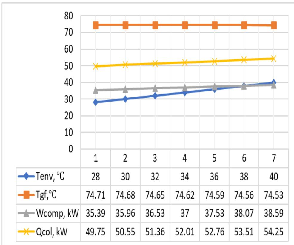
Fig. 9. Relation between  $T_{env}$ ,  $T_{gf}$ ,  $W_{comp}$  and  $Q_{col}$ .
