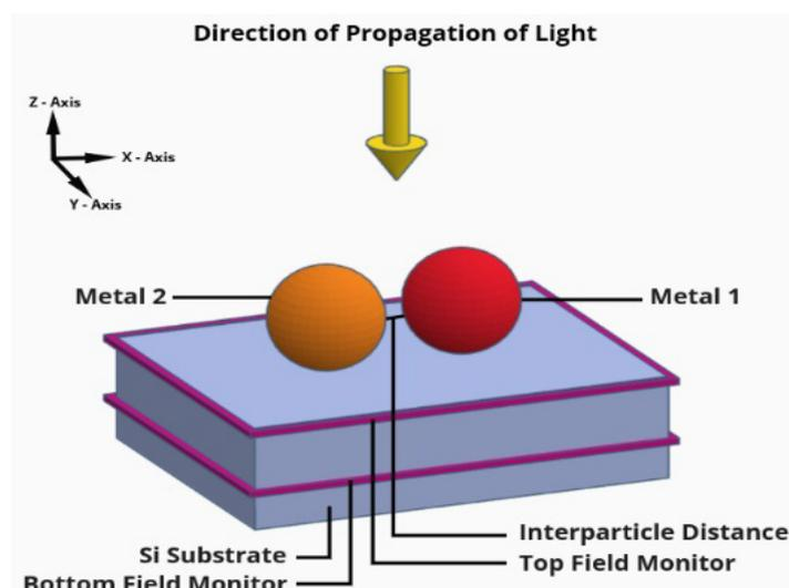
Fig. 6. Simulation schematic showing the plasmonic alloy bimetallic nanoparticle configuration.
