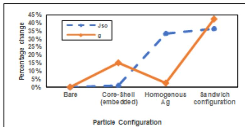
Fig. 4. Optical absorption enhancement ( $g$ ) and short-circuit current density ( $J_{sc}$ ) comparison between different nanostructure configurations with respect to that of bare Silicon substrate [12].
