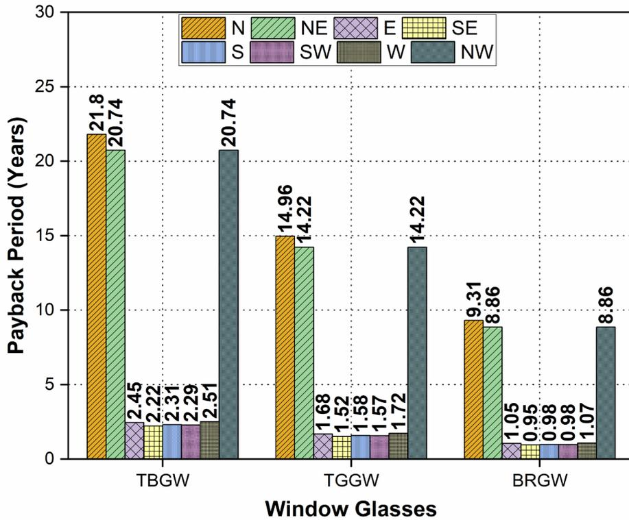
Fig. 8. Payback period of various window glazing.
