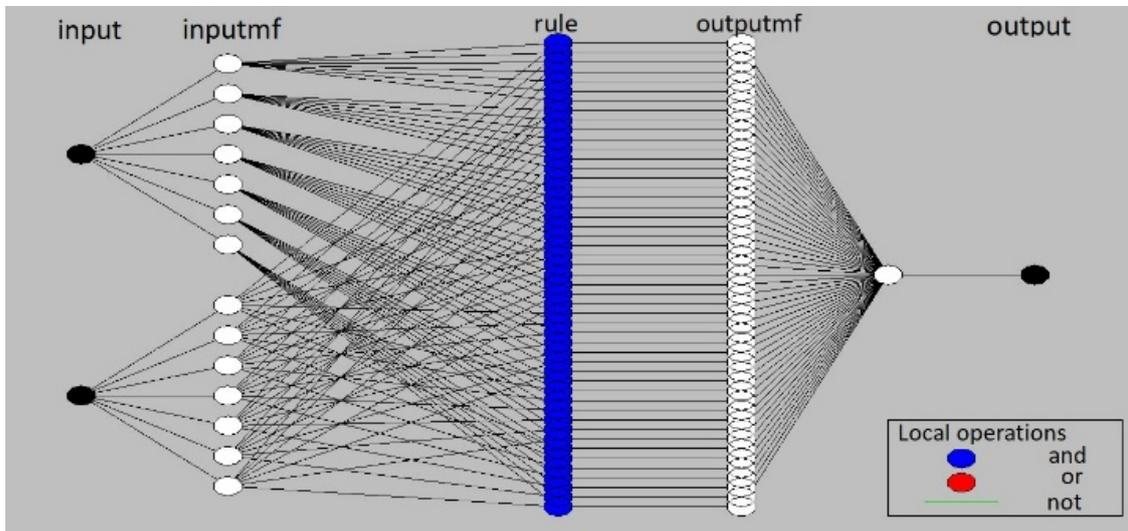
Fig. 14. ANFIS structure showing input(s) and output.
